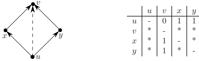
Figure 1: The diamond structure and its adjacency matrix. According to the definition, the solid arcs must be present and the dashed arc must be absent. All other arcs may or may not be present. In the adjacency matrix, the endpoints of each vertex’ outgoing arcs are determined by its row. Stars represent wildcards, that is, these entries do not matter for the definition.
